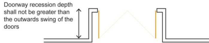
Figure 25. Doorway Recession Regulations
