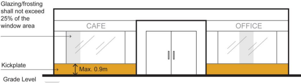
Figure 24. Building Façade Regulations
